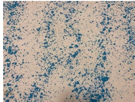
Fig 4. Light Coverage – Splatter Application
