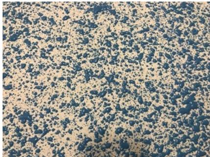
**Fig 3. Correct Coverage – Splatter Application**
