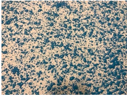
Fig 3. Correct Coverage – Splatter Application
