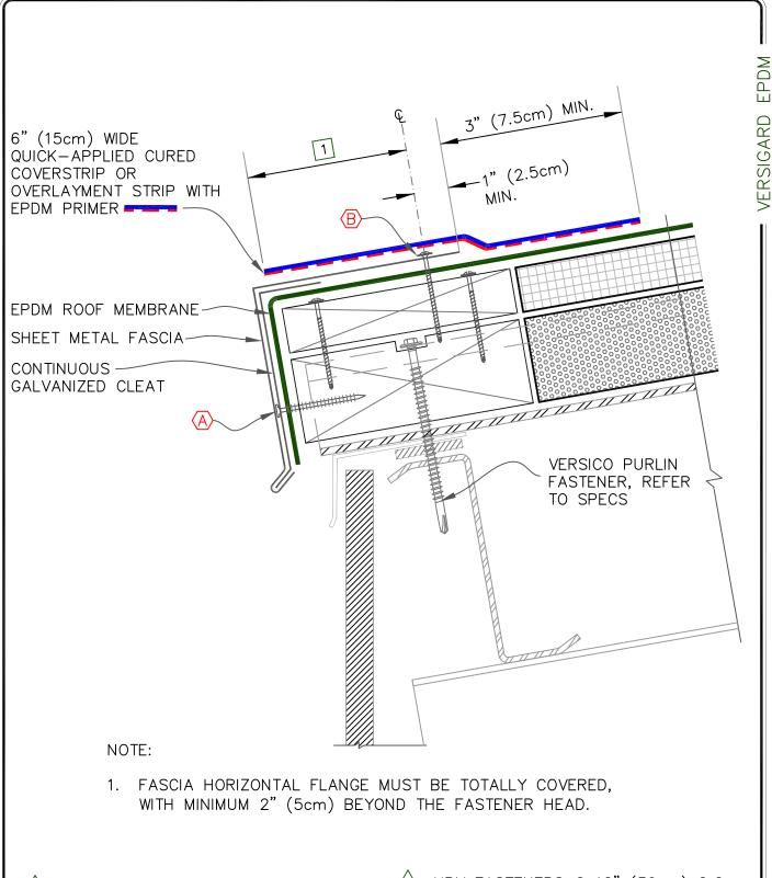
1-1/2" (38mm) RING SHANK NAILS @ B HPV FASTENERS @ 12" (30cm) O.C. 6" (15cm) O.C. MAXIMUM
