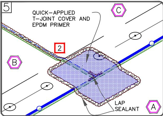
APPLY QUICK-APPLIED T-JOINT COVER OR 6" (15cm) WIDE SECTION OF QUICK-APPLIED UNCURED FLASHING CENTERED OVER THE INTERSECTING POINT OF THE LEADING EDGES OF THE FIELD SPLICE INTERSECTION AS SHOWN.
