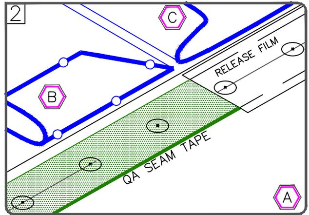
FOLD SHEETS BACK AS SHOWN. APPLY EPDM PRIMER TO THE SPLICE AREA ON BOTH SURFACES AND ALLOW TO FLASH-OFF. APPLY QA SEAM TAPE WITH RELEASE FILM ALIGNED WITH PRE-MARKED LINE.
