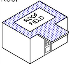
INSTALL PERIMETER SHEETS OVER THE ENTIRE OVERHANG AREA, EXTENDING ONTO THE MAIN ROOF DECK WHEN AT THE SAME LEVEL AS SHOWN.
