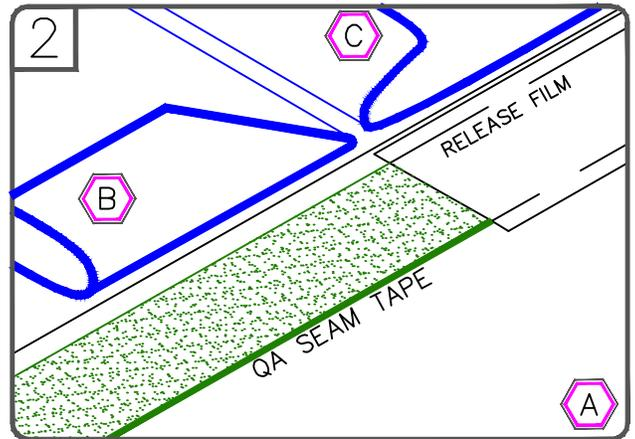
FOLD SHEETS BACK AS SHOWN. APPLY EPDM PRIMER TO THE SPLICE AREA ON BOTH SURFACES AND ALLOW TO FLASH-OFF. APPLY QA SEAM TAPE WITH RELEASE FILM ALIGNED WITH MARKED LINE.
