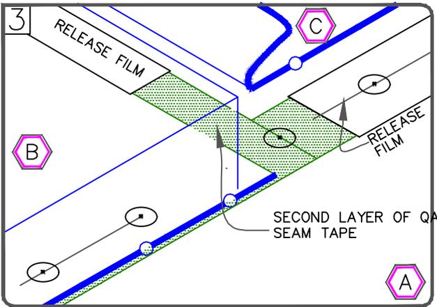
SPLICE SHEET B TO SHEET A AND APPLY SECOND PIECE OF QA SEAM TAPE BETWEEN SHEET B AND C. TRIM RELEASE FILM AS SHOWN.
