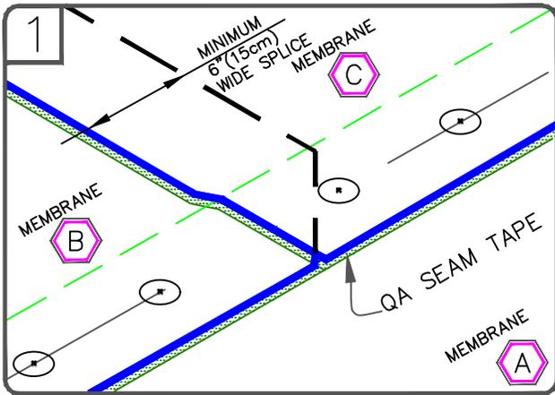
POSITION MEMBRANE TO ALLOW AN APPROXIMATE 7" (17.5cm) OVERLAP. THE PRE-MARKED LINE ON THE MEMBRANE EDGE CAN BE USED AS A GUIDE FOR TAPE PLACEMENT.
