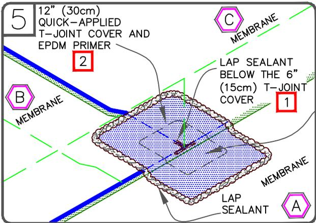
APPLY 6" (15cm) QUICK-APPLIED T-JOINT COVER AND 12" (30cm) QUICK-APPLIED T-JOINT COVER OR QUICK-APPLIED UNCURED CENTERED OVER THE INTERSECTING POINT OF THE LEADING EDGES OF THE FIELD SPLICE INTERSECTION AS SHOWN.
