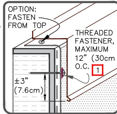
VERSICO FASTENER & SEAM PLATES, MAX. 12" (30cm) O.C.
