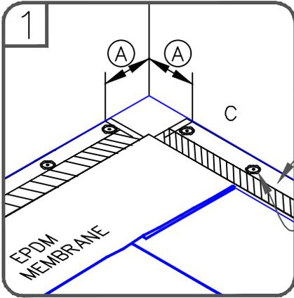
6" (15cm) WIDE QUICK-APPLIED RTS (MAY BE FASTENED INTO VERTICAL SUBSTRATE)
