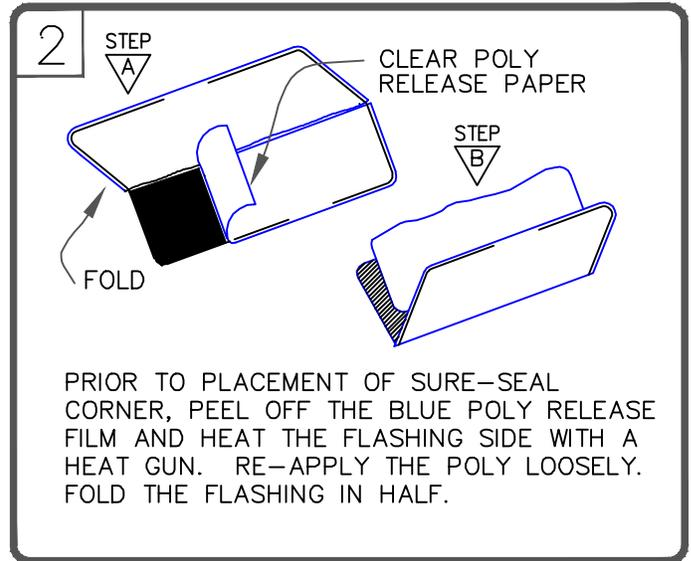
PRIOR TO PLACEMENT OF SURE-SEAL CORNER, PEEL OFF THE BLUE POLY RELEASE FILM AND HEAT THE FLASHING SIDE WITH A HEAT GUN. RE-APPLY THE POLY LOOSELY. FOLD THE FLASHING IN HALF.
