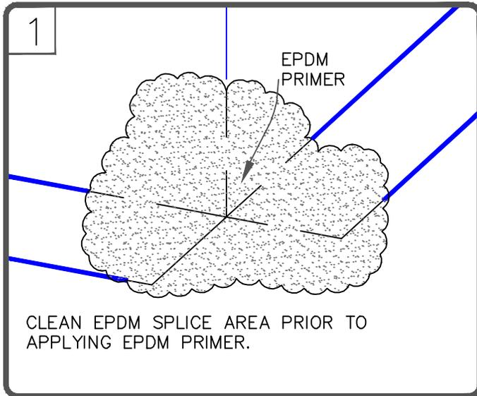
CLEAN EPDM SPLICE AREA PRIOR TO APPLYING EPDM PRIMER.
