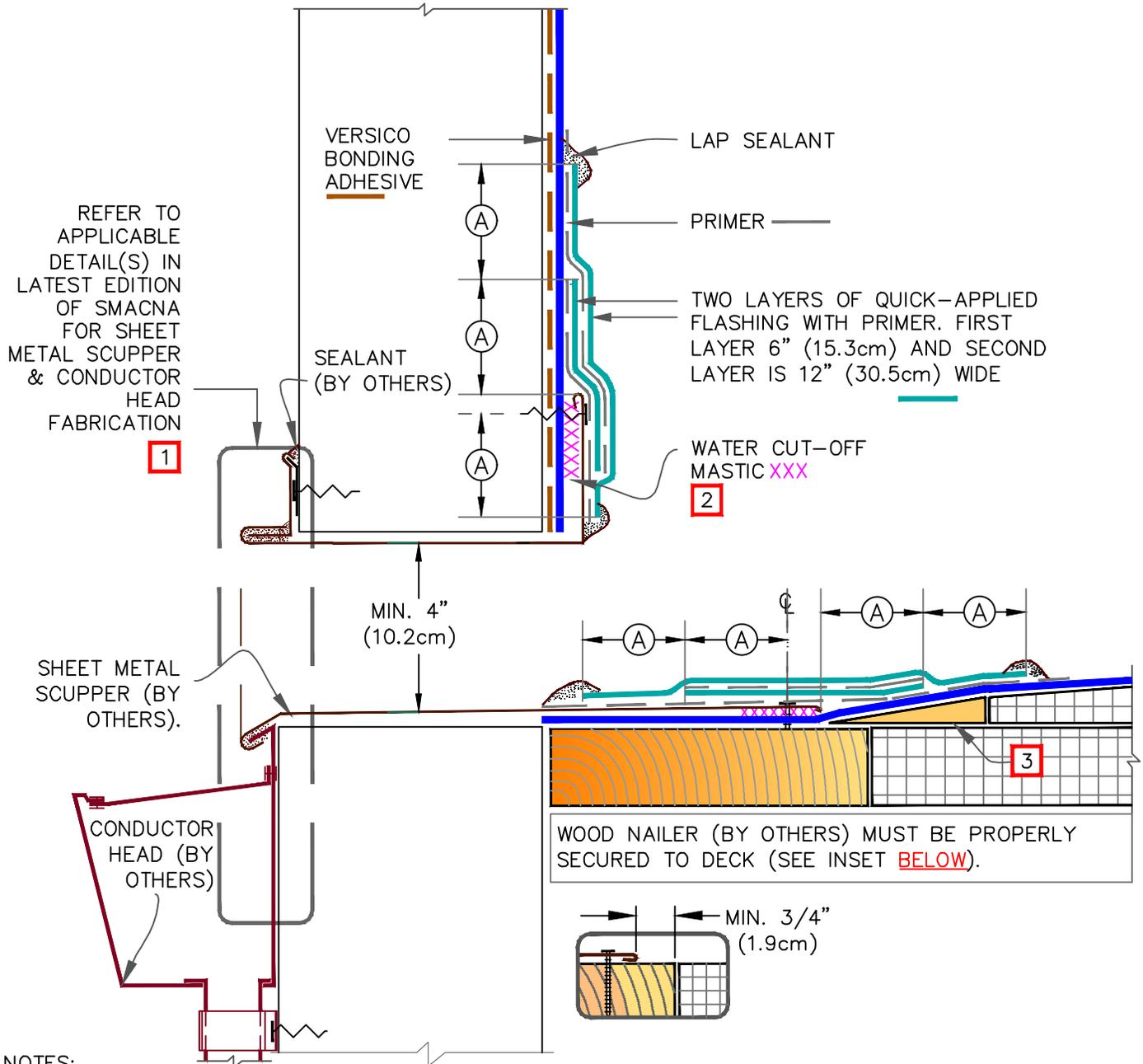
1. METAL SCUPPER BOX MUST HAVE CONTINUOUS FLANGES WITH ROUNDED CORNERS, SOLDER ALL SCUPPER SEAMS AIR & WATER-TIGHT.
