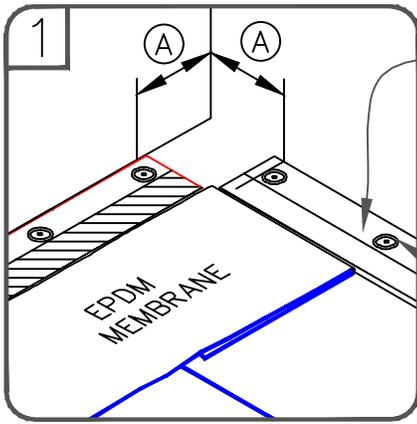
6" (15cm) QUICK-APPLIED RTS (MAY BE FASTENED INTO VERTICAL SUBSTRATE)
