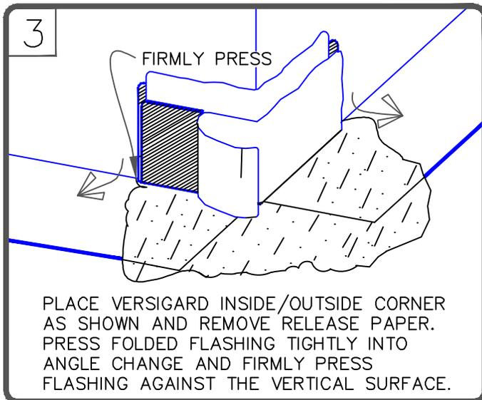
PLACE VERSIGARD INSIDE/OUTSIDE CORNER AS SHOWN AND REMOVE RELEASE PAPER. PRESS FOLDED FLASHING TIGHTLY INTO ANGLE CHANGE AND FIRMLY PRESS FLASHING AGAINST THE VERTICAL SURFACE.
