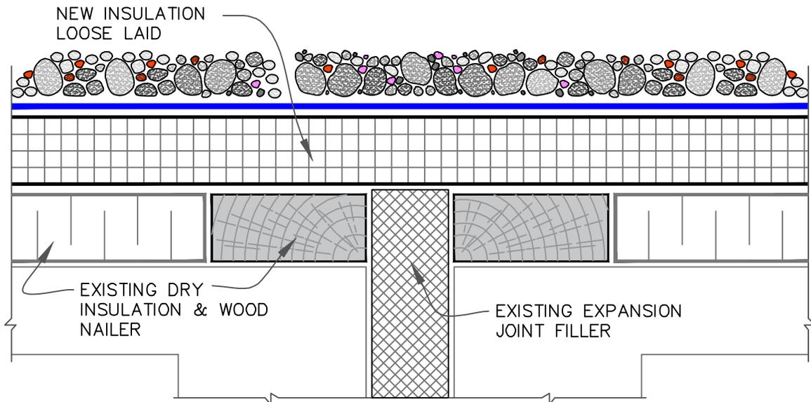
**B** REROOFING OR RECOVER OF EXISTING ROOF
