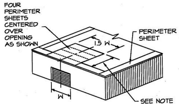
3) As an option to the above perimeter securement, a fully adhered membrane section may be used in lieu of the mechanically attached membrane at large openings in accordance with the Versico Specification for the VersiGard (black and white) Fully Adhered Roofing System.
