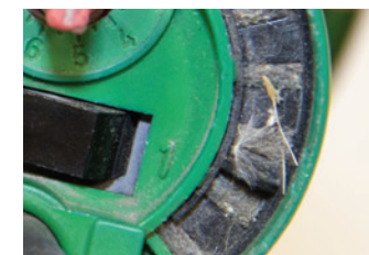
DIRT AND DEBRIS IN INTAKE
