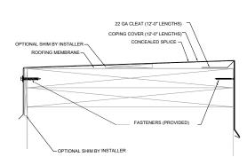
Versico's VersiTrim One Coping was developed as a cost-effective prefabricated solution. VersiTrim One Coping is provided in 12' lengths with pre-punched holes for provided fasteners which simplifies the installation process and ensures a proper fit.
