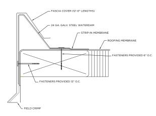
Versico's VersiTrim Crimp-On Fascia offers a canted cleat design creates a water dam at the perimeter of the roof and can also help to keep stone in place on ballasted roofs. Dual attachment points on both the face and horizontal surface allow for added flexibility when accommodating roof irregularities.
