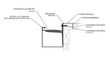
Versico's VersiTrim WR Gutter system incorporates 1" wide extruded internal gutter brackets for strength and support. The system has been engineered to meet ANSI/SPRI GT-1 requirements for wind resistance and is available with 3 distinct looks to fit any building: box style, chamfer style, and offset.
