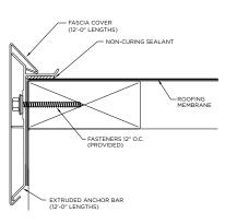
Versico's VersiTrim EX Snap-On Fascia is a two-piece assembly that combines superior performance, attractive appearance, and easy installation. This product eliminates the need for stripping-in or heat-welding and provides the maximum available protection against wind damage. VersiTrim EX Snap-On Fascia is also available in extended face sizes (up to 13") and canted cleat versions.
