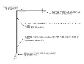
Versico's VersiTrim Drip Edge is a two-part assembly that consists of an L-shaped continuous cleat and a decorative cover with pre-slotted fastening holes on the roof flange. Once the cleat and cover are fastened, the drip edge can be stripped-in using Versico Pressure-Sensitive Cover Strip and Primer.
