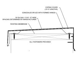
Versico's VersiTrim CF Snap-On Coping is a three piece coping system consisting of coping clips, hidden splice plates, and a snap on coping cap that can be used to cap almost any parapet.
