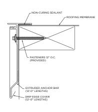
Versico's VersiTrim EX Drip Edge features a patented low-profile extruded aluminum anchor bar and a non-penetrating snap on design that eliminates the need for stripping-in or heat-welding.
