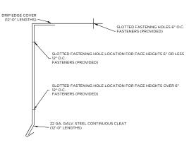
Versico's VersiTrim TPO and PVC-Coated Drip Edge features an L-shaped continuous cleat with pre-slotted fastening holes for ease of installation. VersiTrim TPO Coated Drip Edge is manufactured in 12' lengths while the VersiTrim PVC Coated Drip Edge is manufactured in 10' lengths.
