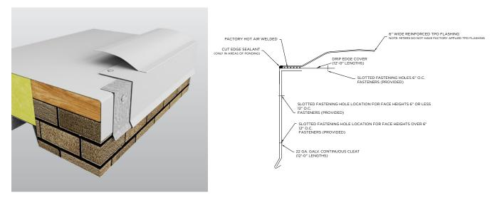
Versico's VersiTrim TPO & PVC Skirted Drip Edge features a 60-mil, 6"-wide, factory-heat-welded TPO or PVC membrane flashing skirt for a quicker installation and a high-quality, consistent weld between the coated metal and the flashing material. VersiTrim TPO & PVC Skirted Drip Edge feature pre-slotted fastening holes that allow for proper thermal movement of materials.
