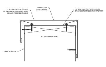
Versico's VersiTrim Gold Coping utilizes a full snap-on design and features a heavy-duty 16-gauge galvanized steel cleat for increased wind resistance. All VersiTrim Copings come with 8" concealed splices with dual non-curing butyl sealant strips to prevent water infiltration and allow for thermal movement at joints.
