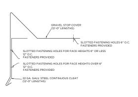
Versico's VersiTrim Gravel Stop's two-part assembly consists of an L-shaped continuous cleat and a decorative cover with pre-slotted fastening holes on the roof flange. Once the cleat and flange are fastened, the gravel stop can be stripped-in using Versico's Pressure-Sensitive Cover Strip and Primer. The rise at the edge of the roof is customizable (minimum of ½" high).
