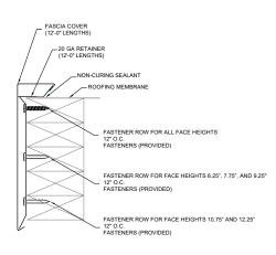
Versico's VersiTrim CF Snap-On Fascia is a two-part assembly that includes a formed steel retainer cleat and a decorative snap-on cover. The simple design allows for fast installation while still delivering excellent performance.
