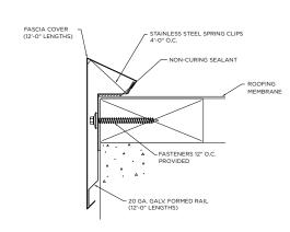
Versico's VersiTrim One Fascia is a cost-effective, high-performance product with a minimal lead time. This product eliminates the need for stripping-in or heat-welding, is manufactured and tested to meet ANSI/SPRI ES-1 standards, and is Factory Mutual approved.
