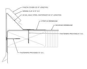
Versico's VersiTrim Snap-On Canted Fascia features a snap-on cover that eliminates crimping, substantially reducing installation time. The canted cleat design creates a water dam at the perimeter of the roof and can also help to keep stone in place on ballasted roofs. Dual attachment points on both the face and horizontal surface allow for added flexibility when accommodating roof irregularities.
