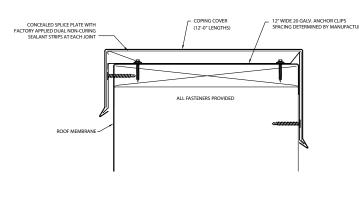
Versico's VersiTrim Snap-On Coping utilizes a full snap-on design to ensure long-term positive attachment and ease of installation. It is custom-fabricated to meet your exact job requirements.
