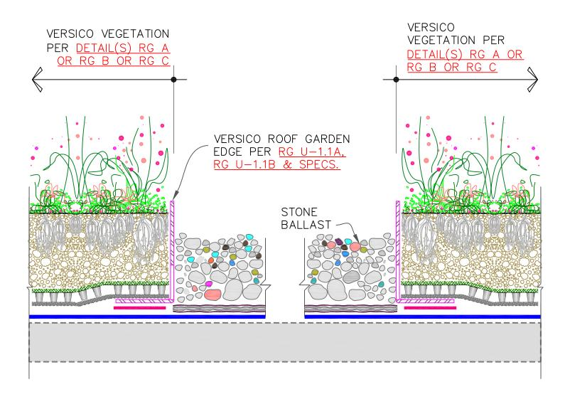
1. FOR ALTERNATE DETAILS SEE DETAILS RG 12.3, RG 12.5 OR RG 12.7
