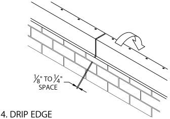
PROVIDED FASTENERS. LAP CLEAT 1" AT JOINTS.
