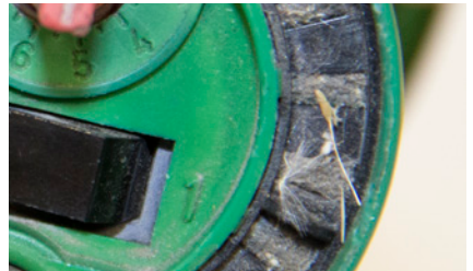
Dirt and debris in intake
