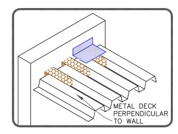
INSTALL PRESSURE-SENSITIVE FLASHING OR 725TR AIR & VAPOR BARRIER ON TOP FLUTES OF METAL DECK & WALL
