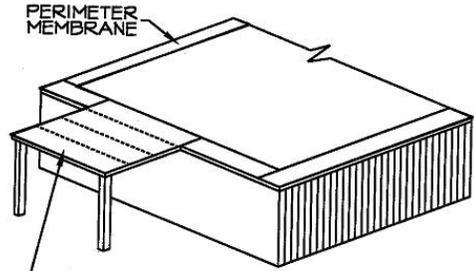
INSTALL PERIMETER SHEETS OVER THE ENTIRE OVERHANG AREA EXTENDING ONTO THE MAIN ROOF DECK WHEN AT THE SAME LEVEL AS SHOWN.
