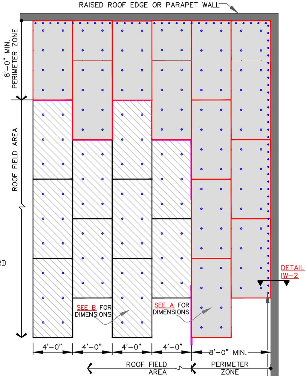
MEMBRANE FASTENED MINIMUM 12" O.C. AT ANGLE(S) CHANGES. FOR ADDITIONAL INFORMATION SEE DETAIL IW-2
