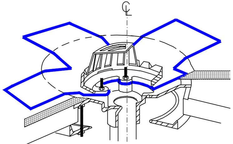
EXTEND PVC MEMBRANE ONTO MEMBRANE SECTION POSITIONED AT DRAIN SUMP AND CUT AS SHOWN TO LAY FLAT IN SUMP. HOT AIR WELD A MINIMUM OF 1- 1/2" (4cm) COMPLETELY SURROUNDING AREA.
