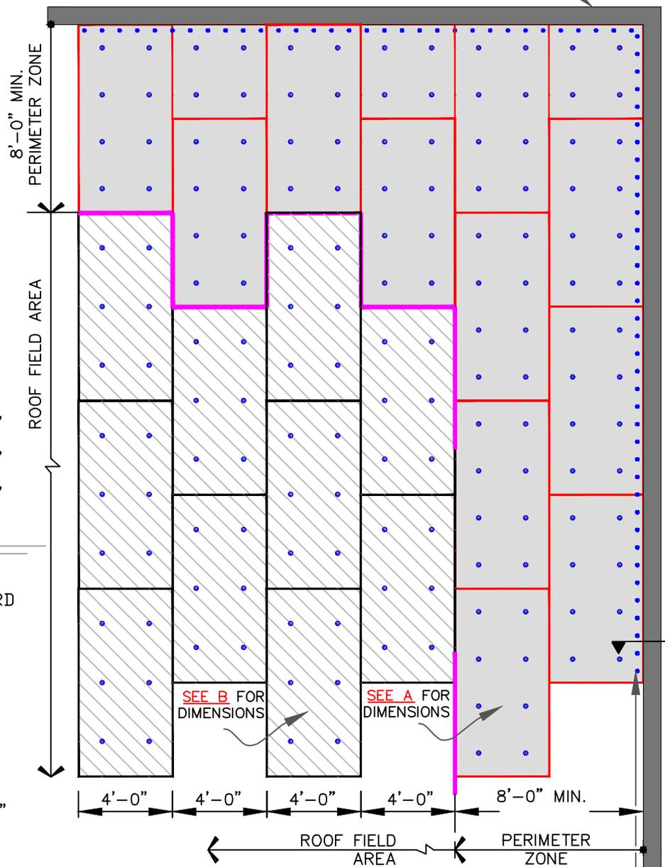
MEMBRANE FASTENED MINIMUM 12" O.C. AT ANGLE(S) CHANGES. FOR ADDITIONAL INFORMATION SEE DETAIL RB-2
