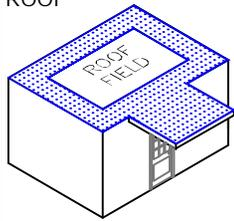
INSTALL PERIMETER SHEETS OVER THE ENTIRE OVERHANG (PROJECTION ROOF) AREA, EXTENDING ONTO THE MAIN ROOF DECK WHEN AT THE SAME LEVEL AS SHOWN.
