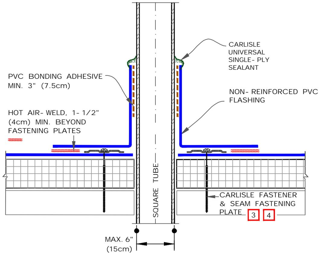
**FASTENER TYPES ON MECHANICALLY FASTENED ROOF ASSEMBLY**
