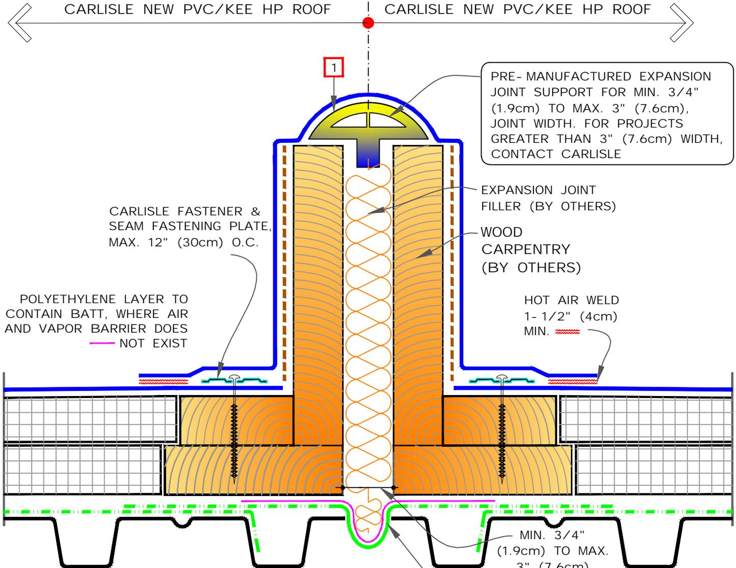
PRE-MANUFACTURED EXPANSION JOINT SUPPORT FOR MIN. 3/4" (1.9cm) TO MAX. 3" (7.6cm), JOINT WIDTH. FOR PROJECTS GREATER THAN 3" (7.6cm) WIDTH, CONTACT CARLISLE
