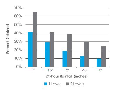
During a heavy, one-inch rainfall, over 6,200 gallons of water would fall onto a 10,000 ft² roof. Versico's Ballasted Stormwater Retention System using two layers of moisture retention mat could retain up to 67%, or 4,177 gallons. This provides serious relief to local stormwater and sewer systems, while only adding a little over 3 lbs of weight per square foot of roof area.
